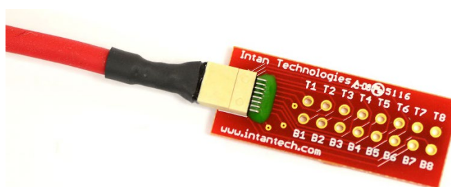
Figure 2. Stim SPI cable adapter board plugged into RHS Stim SPI interface cable.
