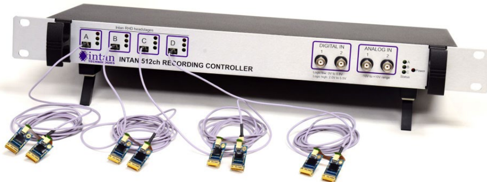
Intan RHD Recording Controller (512ch or 1024ch) (up to 1024 amplifier channels using RHD headstages)
